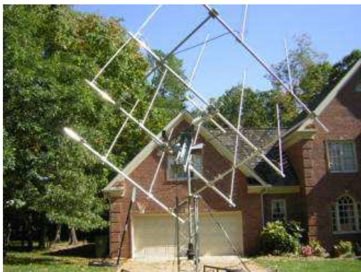
N8CQ 16 yagi portable on trailer with pol. rot.
